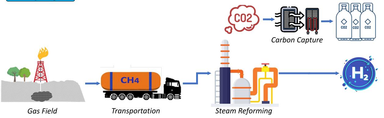
Blue hydrogen is produced mainly from natural gas, using a process called steam reforming, which brings together natural gas and heated water in the form of steam. The output is hydrogen, but carbon dioxide is also produced as a by-product. So, the definition of blue hydrogen includes the use of carbon capture and storage (CCS) to trap and store this carbon.
