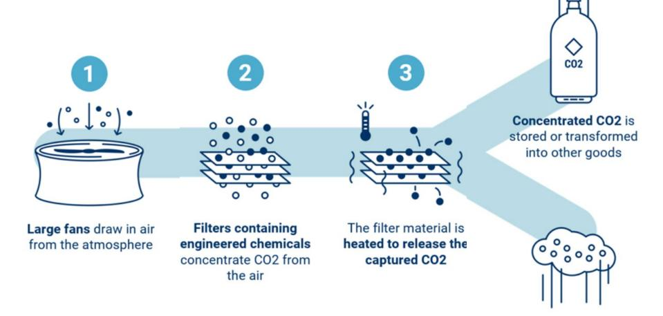
Filtered, CO2-free air is released into the atmosphere
