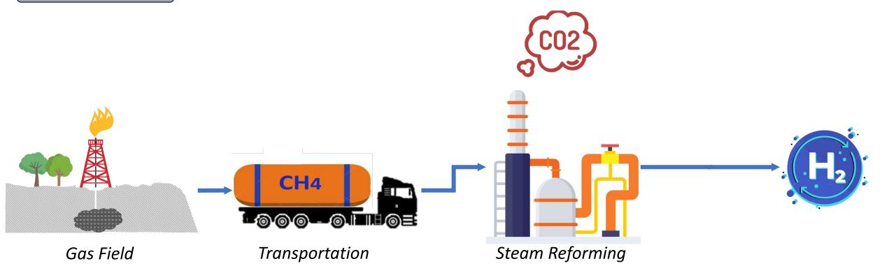
Currently, this is the most common form of hydrogen production. Grey hydrogen is created from natural gas, or methane, using steam methane reformation but without capturing the greenhouse gases made in the process. Grey hydrogen is essentially the same as blue hydrogen, but without the use of carbon capture and storage.
