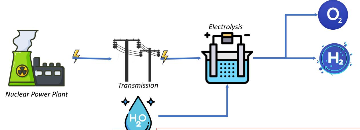
Pink hydrogen is generated through electrolysis powered by nuclear energy. Nuclear-produced hydrogen can also be referred to as purple hydrogen or red hydrogen.
