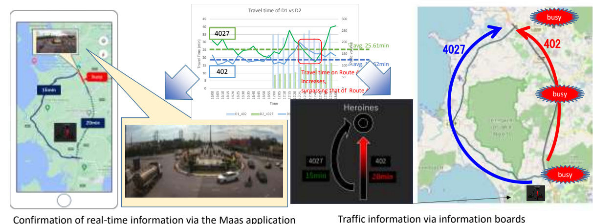
Figure 2: A Method of Providing Traffic Information Using Combined Analysis of CCTV and Probe Data
