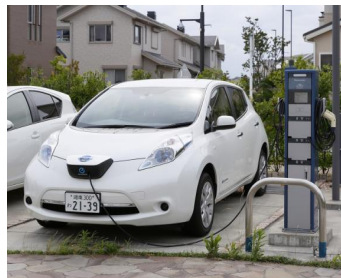
Two EVs are reserved. In case of an emergency, the V2H system supplies electricity to the assembly room, etc.
