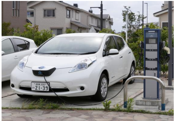
Two EVs are reserved. In case of an emergency, the V2H system supplies electricity to the assembly room, etc.
