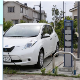
reserved. In case of an emergency, the V2H lies electricity to the assembly room, etc.
